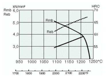
Bend strength of a bar with diameter 5 mm after hardening and tempering to  $560^{\circ}C / 1040^{\circ}F$ , 2x1 h. Rmb = Ultimate bend strength kN/mm<sup>2</sup>,  $\pm 10\%$ Reb = Bend yield strength kN/mm<sup>2</sup>,  $\pm 5\%$ HRC = Hardness  $\pm 1$  HRC
