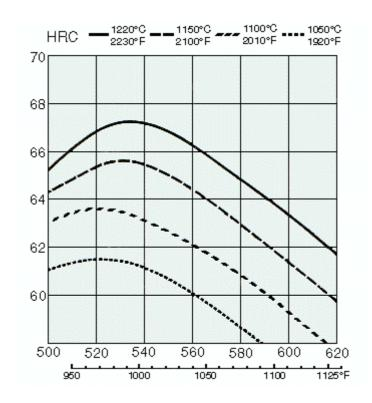
Hardness after hardening, step quenching and tempering 2x1 h of a sample 25 mm Ø.
